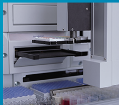
The DSX's robotic arm moves microplates and pipettes all samples and reagents.
